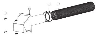
Installation of a fresh air kit is required when installing this stove inside a mobile home (see Owner's Manual). Installation must adhere to all local codes. If after reading these instructions you have any doubt about your ability to complete the installation properly, you must obtain the services of a licensed heating and cooling contractor or certified stove installer.
