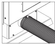
4. Route the flex pipe to the through wall connection and slide the flex pipe over the tail piece. Apply the second hose clamp over the tail piece and tighten.
