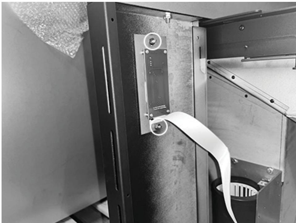
Figure 19: Install control panel.
