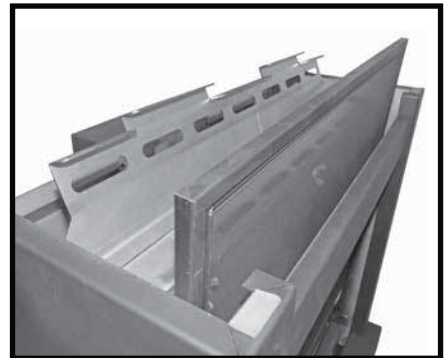
Figure 39: TN24 mesh removal.
