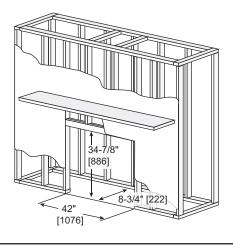
Adjust framing dimensions for interior chase sheathing (such as sheetrock)
