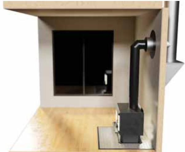
THROUGH THE WALL INSTALLATION
