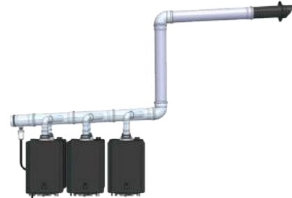
ROOM AIR WITH HORIZONTAL EXHAUST (NEW)
