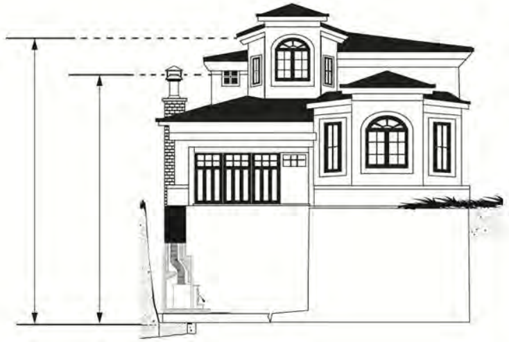
Figure 32: Chimney location in the house
