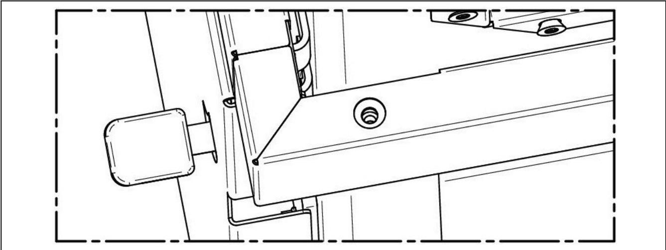
6 - Close the doors and check if the molding is properly aligned with the top and bottom doors (=), as well as with the side moldings (A & B). **See the following steps for adjustment options.**
