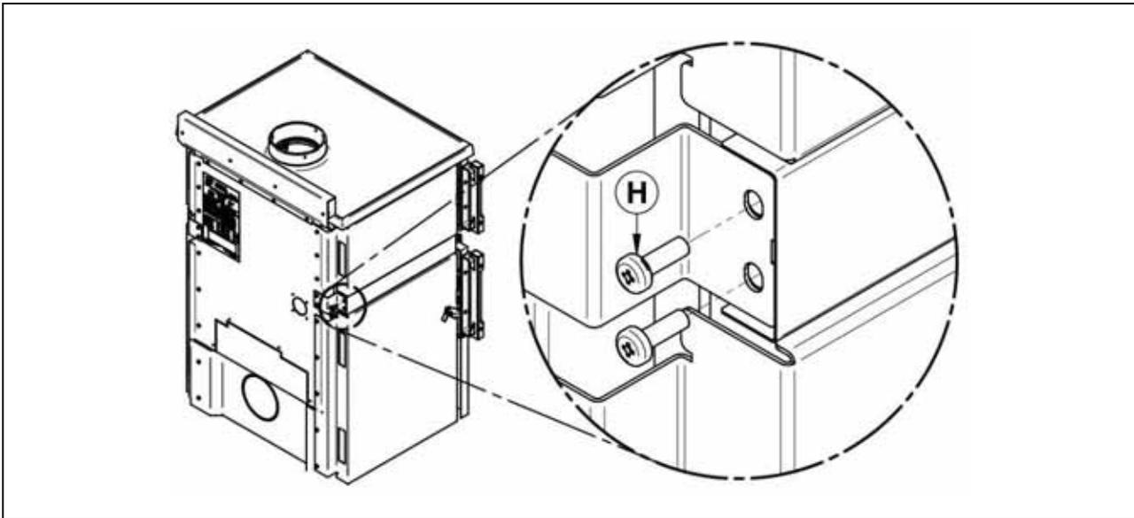
**4** - Adjust the molding so that it is evenly aligned (=) with the decorative sides of the product. Then, tighten the screws (**H**).
