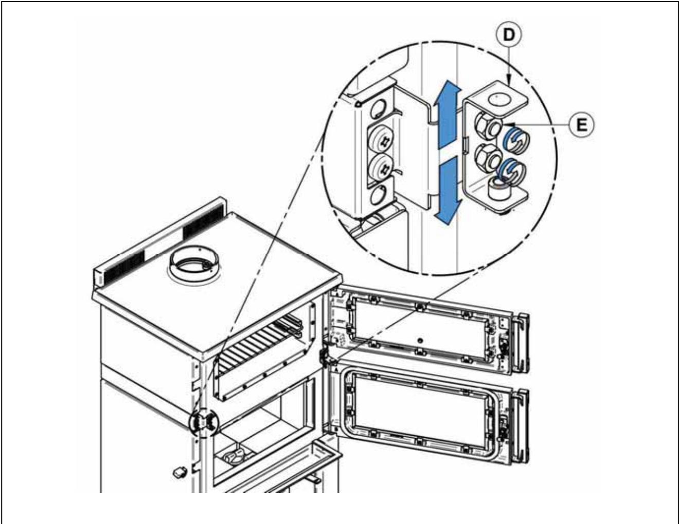
**Option 2** - This adjustment option allows you to adjust the positioning of the central molding and the side moldings.
