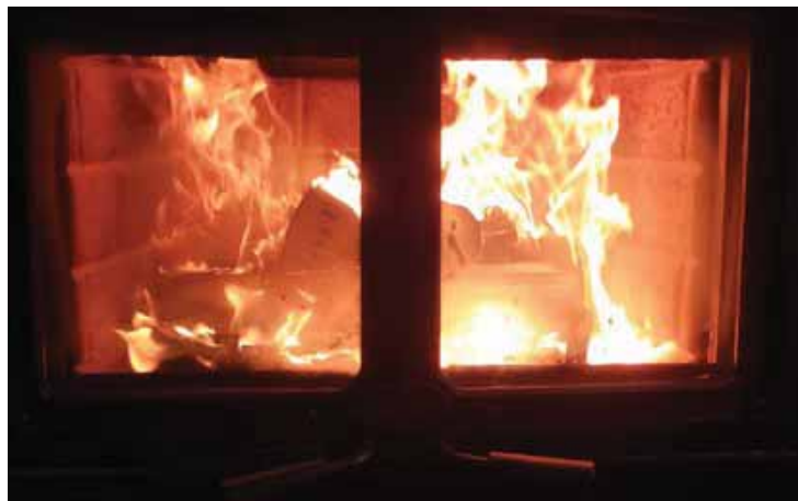
Figure 18: Flames intensity at the beginning of Start-up phase (Door cracked about 1 inch)
