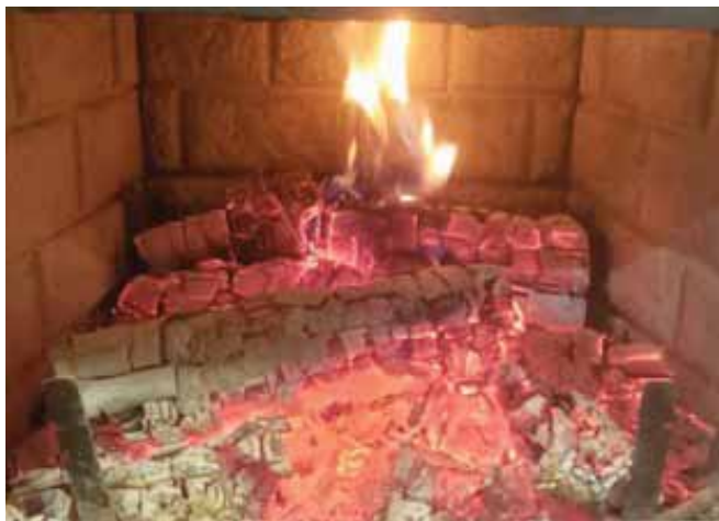
Figure 24: Charcoal bed at the end of High-fire phase
