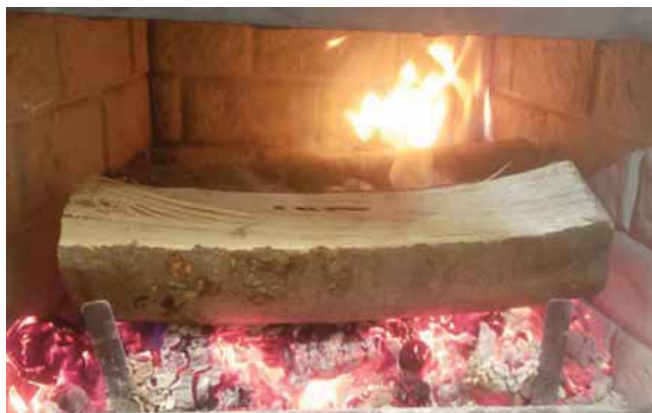
Figure 25: Maintenance-fire load in firebox
