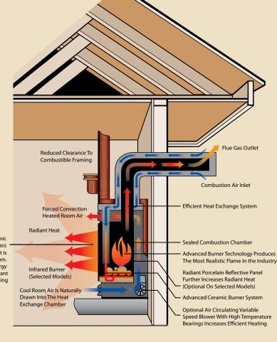
High Heat Ceramic or Tempered Glass increases the radiant heat that is dispersed throughout the room. Save up to 30% on energy costs with radiant heat and Zone Heating
