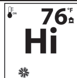
FIGURE 59 Blower at HI
