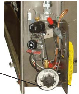
Rear burner control knob
