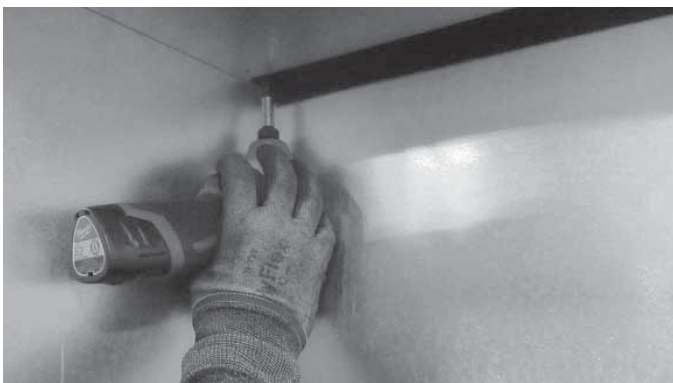
Figure 7.2 - Remove Rear Black Magic Glass Bracket
