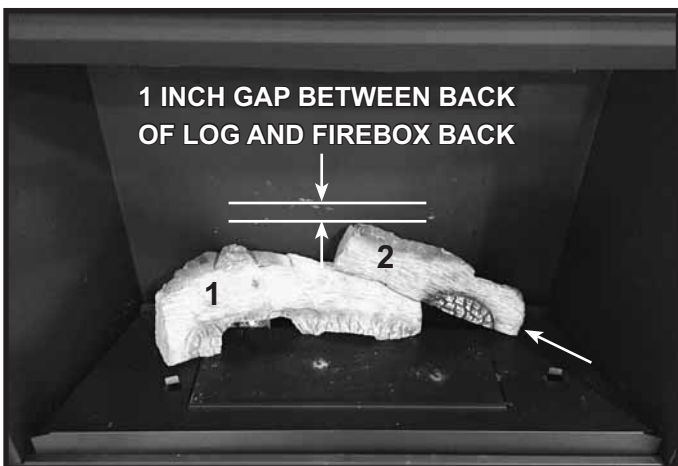
Figure 5. Install Right Rear Base Log
