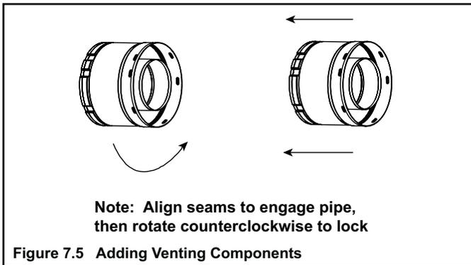
**NOTICE:** When installing a vent system with an HRC termination cap, all pipe system joints shall be sealed using a high temperature silicone sealant (300 °F minimum continuous exposure rating).
