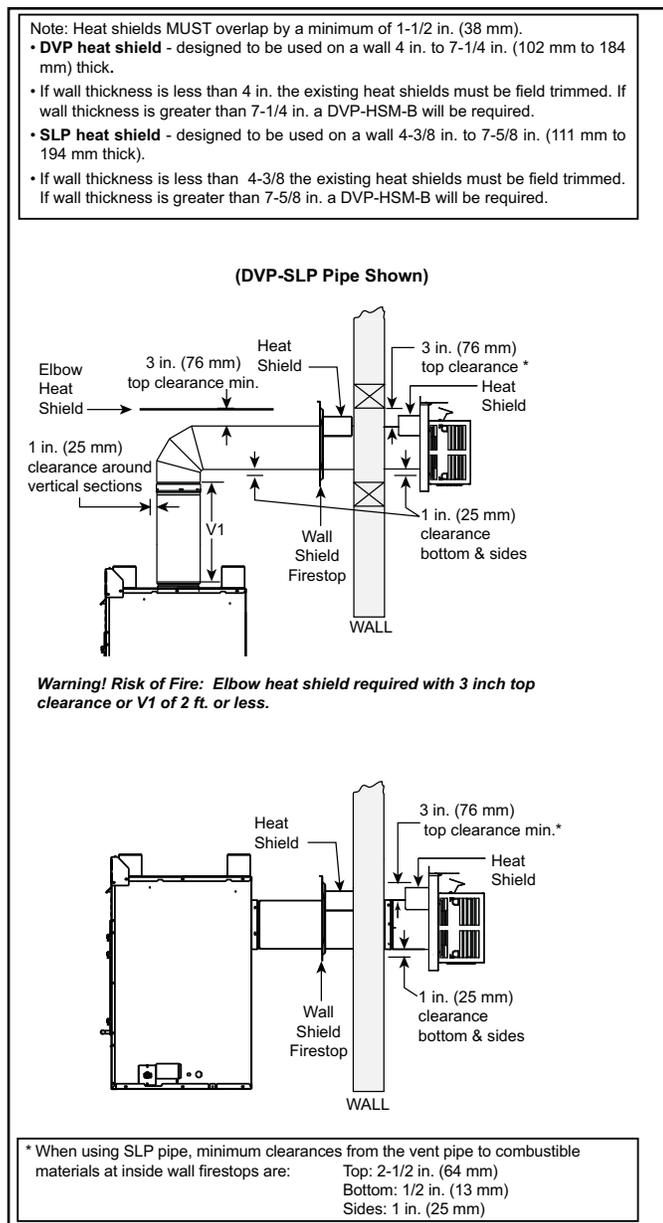
Figure 5.1 Horizontal Venting Clearances To Combustible Materials
