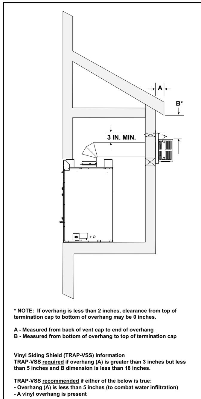
Figure 3.14 Exterior Chase - Minimum Height Requirements
