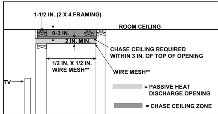
**WARNING! Risk of Fire!** Wire mesh required on bottom of discharge opening (Dimension A) when finished discharge opening is greater than 3 inches. Secure mesh to top of framing.
