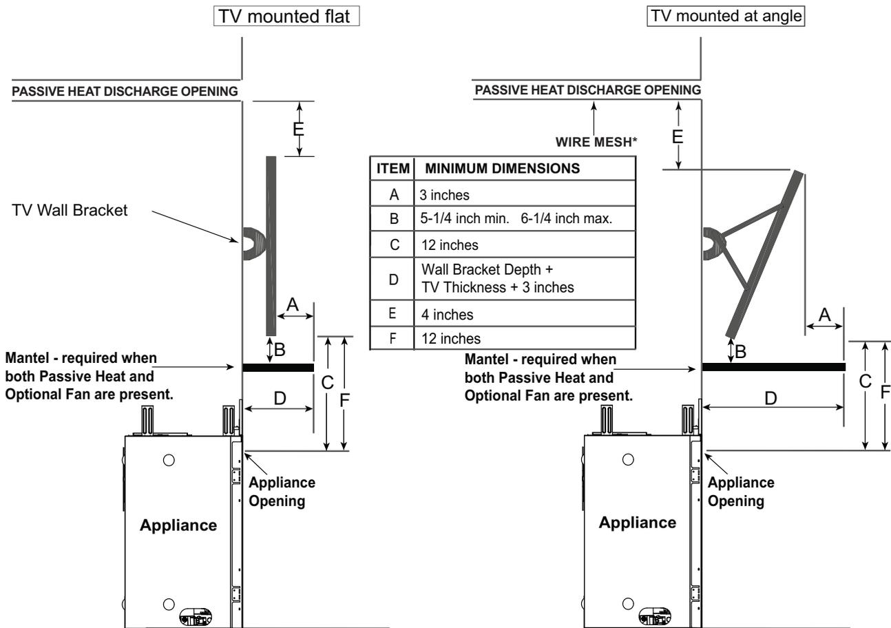
\* Mesh screen required for front discharge or open top discharge passive heat installations with discharge opening of three inches or greater.
