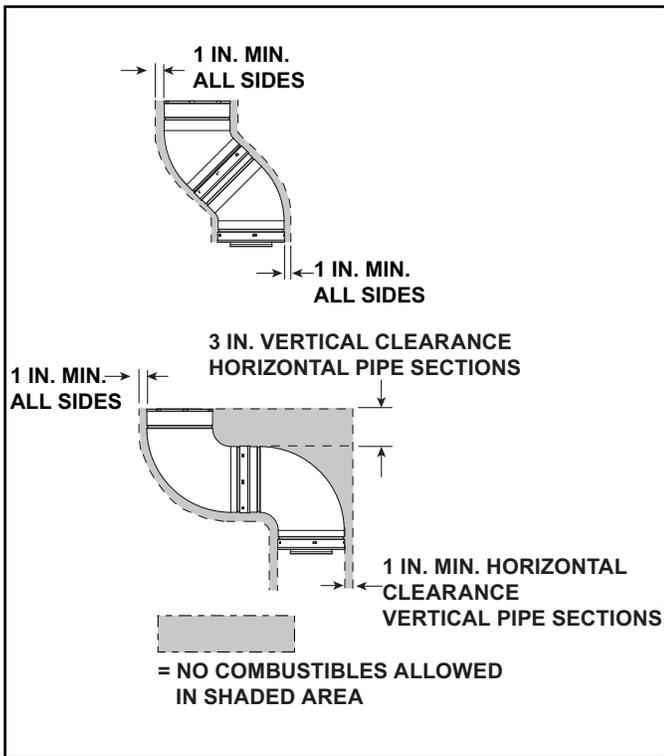
Figure 5.3 Clearances from Vent to Combustible Framing Materials
