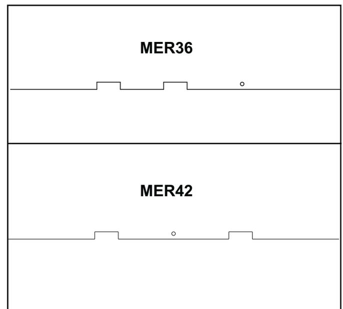
Figure 9.3 Burner Identification
