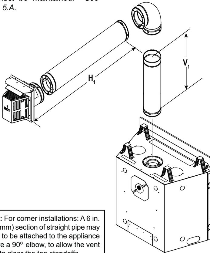
**Note:** For corner installations: A 6 in. (152 mm) section of straight pipe may need to be attached to the appliance before a 90° elbow, to allow the vent pipe to clear the top standoffs.
