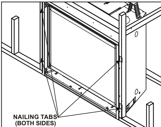
Figure 6.13 Proper Positioning and Securing of an Appliance
