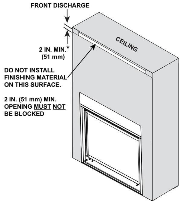
\* = Mesh screen required for front discharge or open top discharge passive heat installations with discharge opening of 3 in. (76 mm) or greater.
