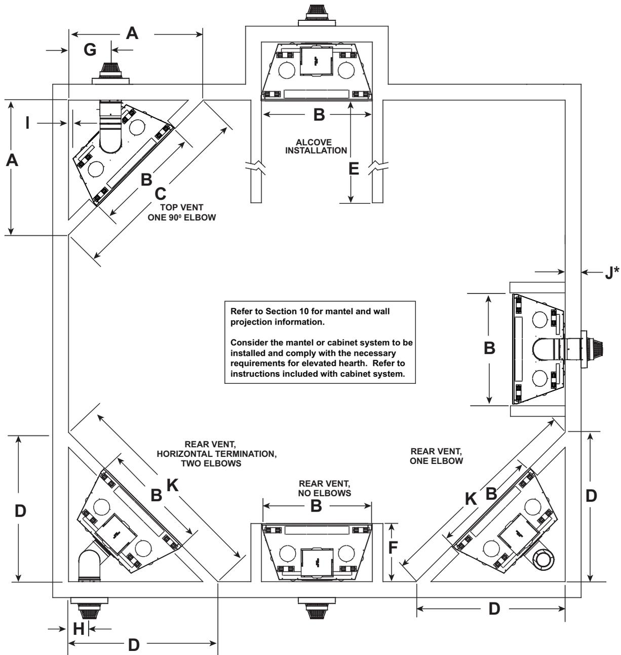
J\* = When exterior wall is constructed from 2 x 4 material, a termination cap with effective length equal to the DVP-TRAP1 is required. See Figure 3.9.
