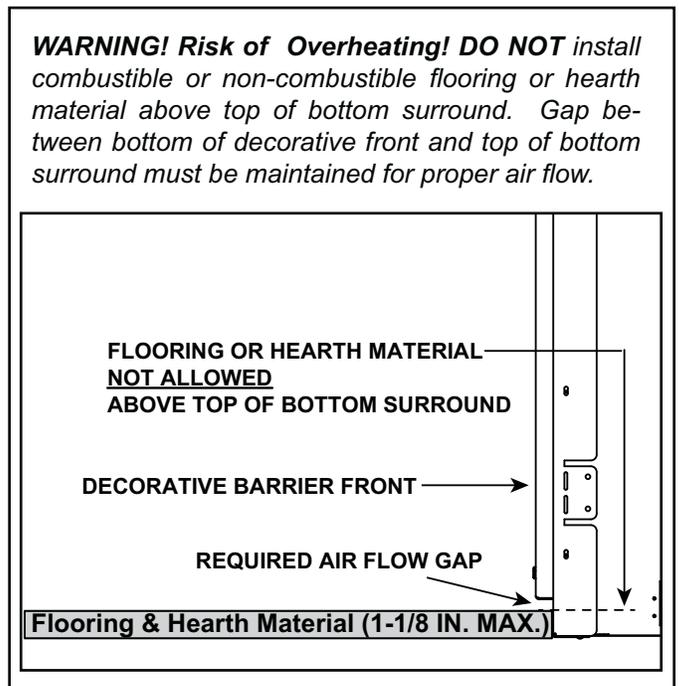
Figure 10.3 Required Air Flow Gap
