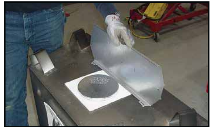
Figure 6.6 Rotate the top heat shield to the vertical position as shown above. The heat shield must remain in the vertical position.
