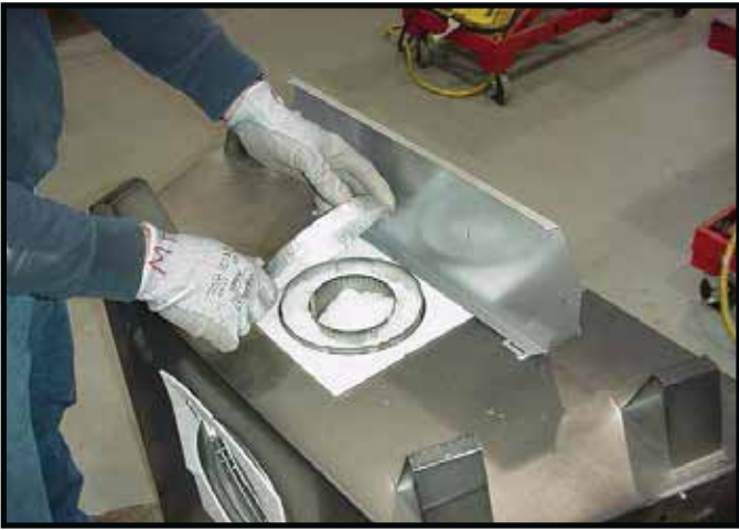
Figure 6.8 Remove the seal cap.
