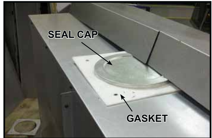
Figure 6.2 Seal Cap and Gasket Location
