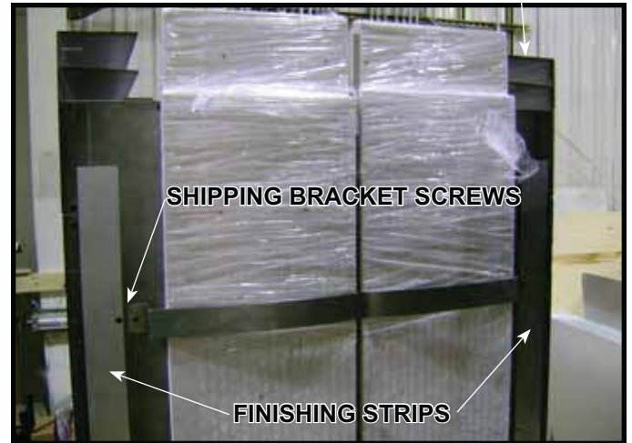
Figure 6.3 Shipping Brackets and Finishing Strip Locations.
