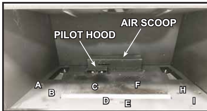
Figure 2. Empty Firebox with Shoulder Screw Locations
