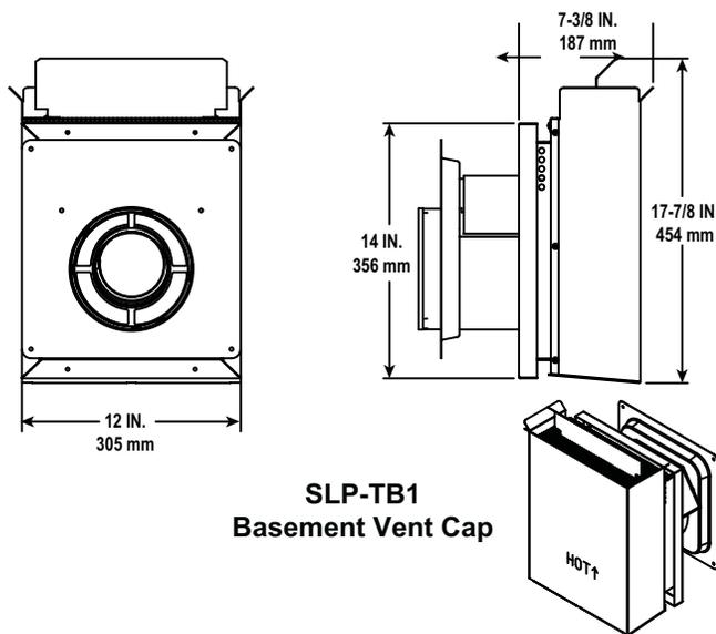
Figure 12.5 Vent Components
