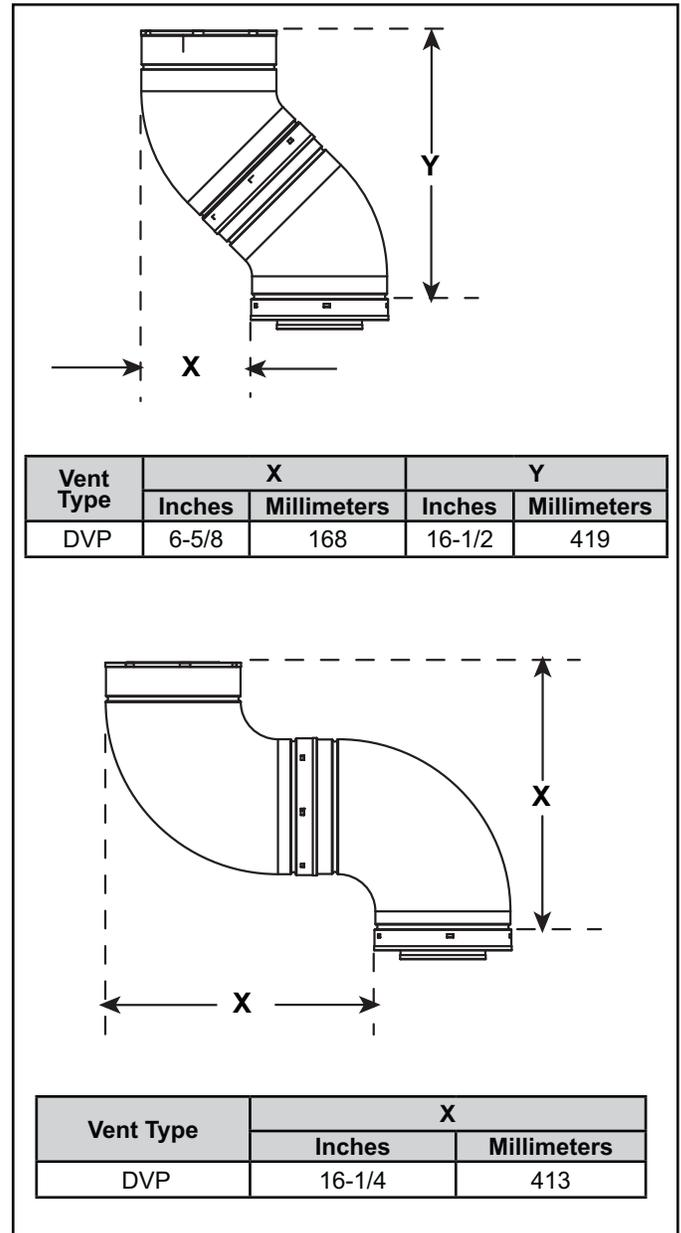
Figure 4.7 Vertical and Horizontal Offset for DVP Elbows
