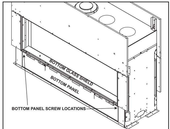
Figure 9.2 Bottom Glass Shield and Bottom Panel Location
