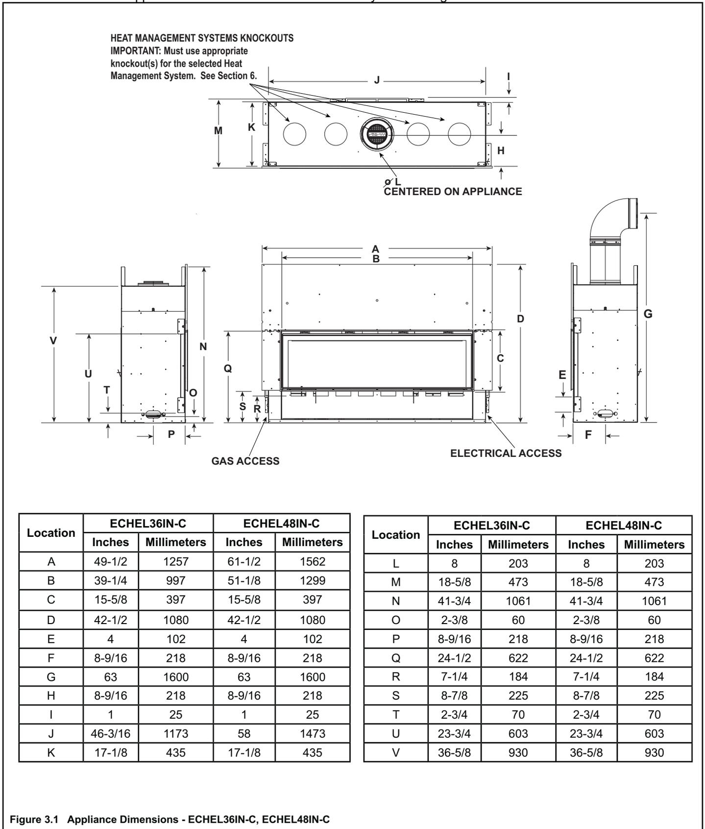
Figure 3.1 Appliance Dimensions - ECHEL36IN-C, ECHEL48IN-C
