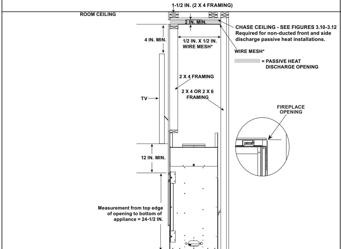
\* Wire mesh required for front discharge or open top discharge passive heat installations with discharge opening of 3 inches or greater.
