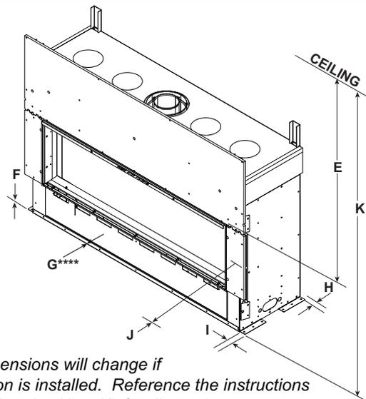
**NOTE:** E & K dimensions will change if Passive Heat option is installed. Reference the instructions included with the Passive Heat Kit for dimensions.
