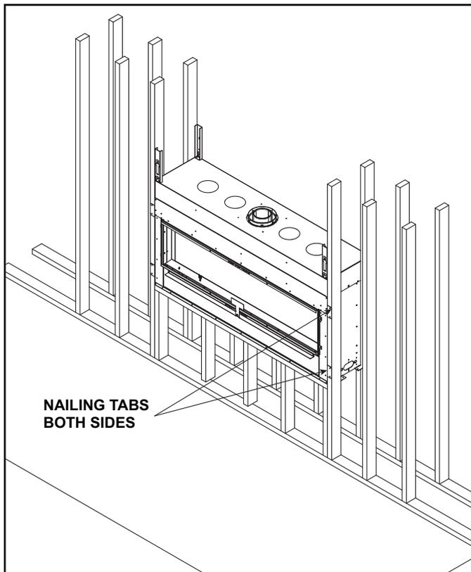
Figure 6.8 Proper Positioning and Securing of an Appliance
