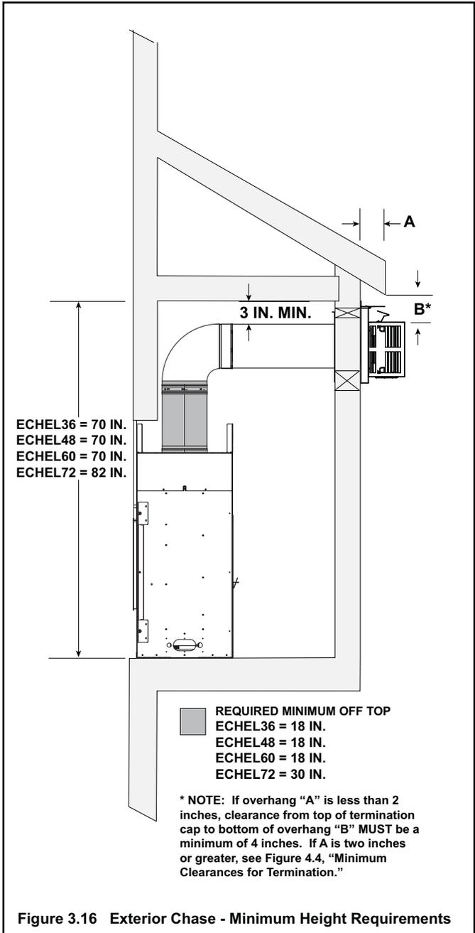
Figure 3.16 Exterior Chase - Minimum Height Requirements
