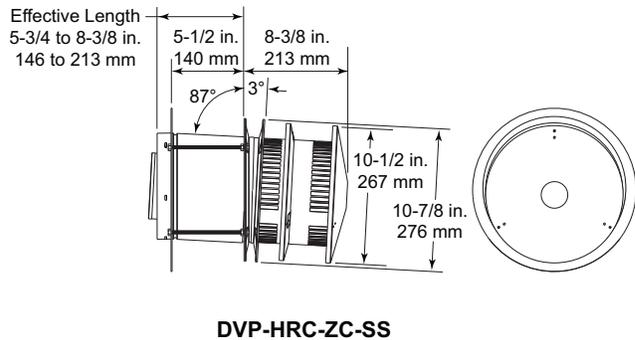
Figure 12.4 DVP Vent Components
