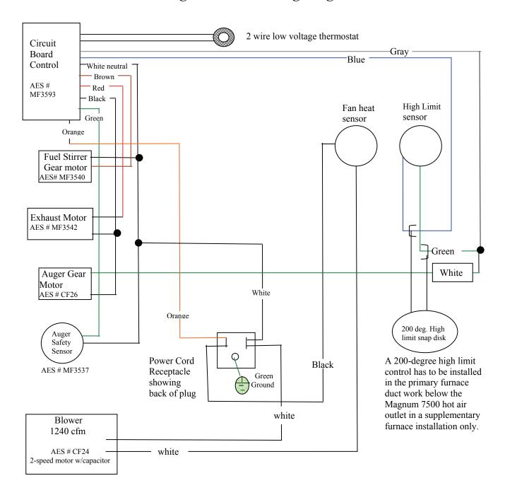
The High limit control is pre-set and does not need to be adjusted. If the furnace is overheating consult your HVAC installer for proper duct installation, pressures and sizing.
