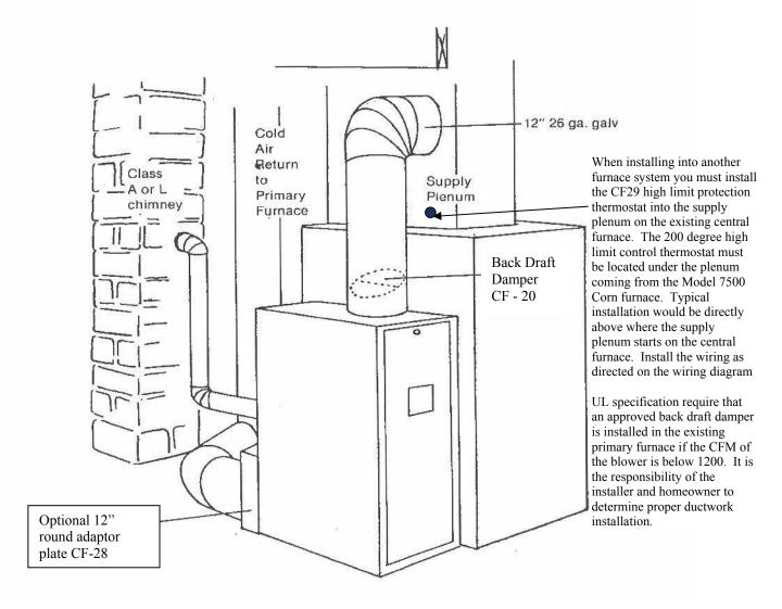
**Add-On Furnace (Supplementary Heat installation)**
