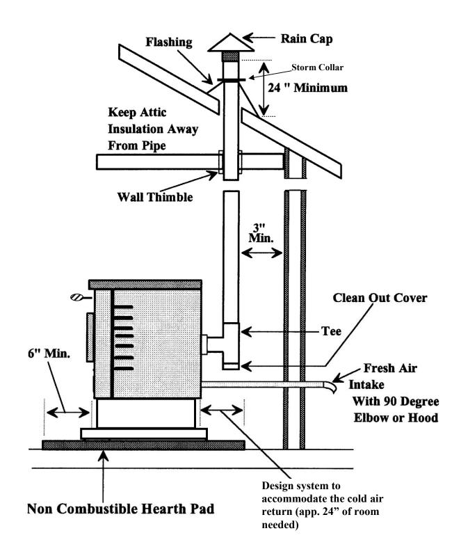
INSIDE VERTICAL PIPE WITH ROOF TERMINATION
