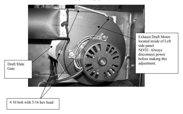
The normal operation of the Magnum would be with the Draft Slide Gate open fully as shown. When the gate is in the fully open position, the plate will be against the mounting plate as shown.
