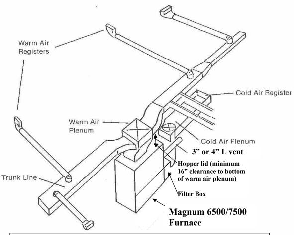
Installation configuration when using the Magnum 6500/7500 furnace as an independent ductwork installation separate from the existing primary furnace. The Magnum Furnace is not intended to be installed as the sole source of heat and is not allowed to be the sole source of heat in most states and building/ insurance codes.
