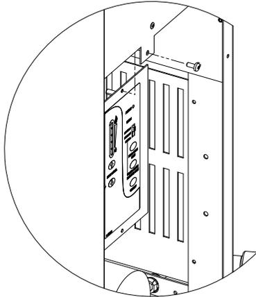
Figure 23: Removing the control panel from the unit
