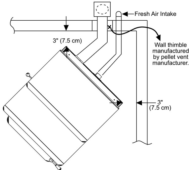
Figure 12: Corner Installation.
