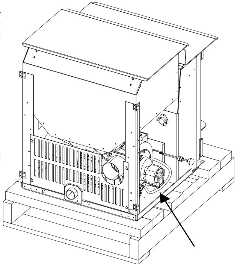
Figure 3: Removing Freestanding Stove From the Pallet.
