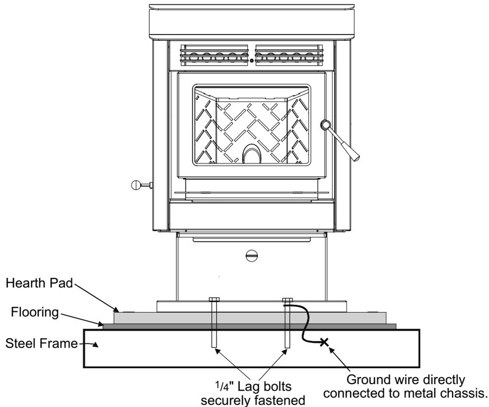
Figure 7: Mobile Home Install Mounting.
