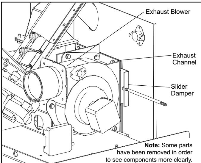
Figure 27: Slider / Damper
