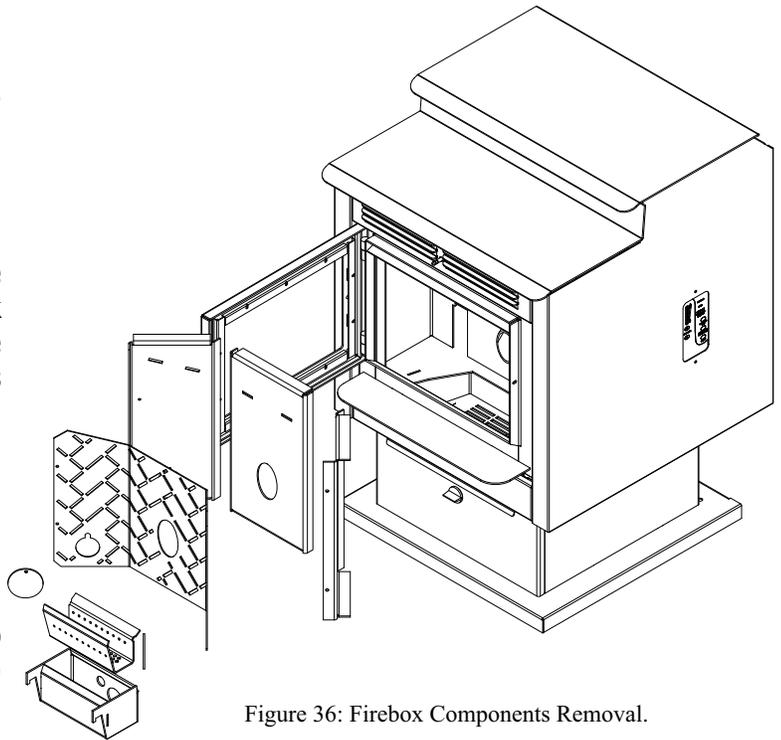
Figure 36: Firebox Components Removal.
