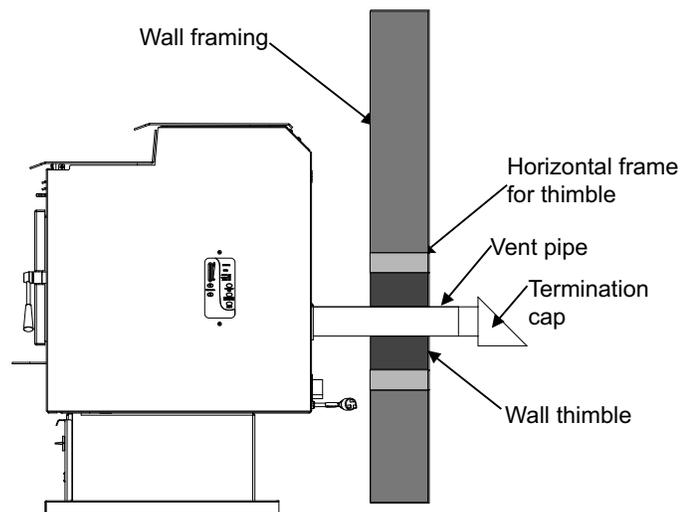
Figure 14: Straight through Wall Installation - Side View.
