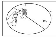
Do not spray any aerosol near heater when in operation. Do not store these elements near appliance.
