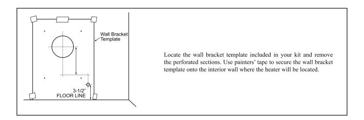
Trace the template flue outlet hole and the gas inlet hole onto the wall. Mark the four (4) wall bracket mounting screw holes onto the wall. The size of the gas inlet hole will depend upon the size of gas pipe coming into the unit. (See page 9, top graphic, items A and B). The center of the gas inlet hole will be located 3-1/2" from the floor line.
