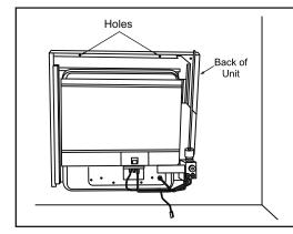
Line up the two (2) screws in the top of the mounting bracket with the holes in the back of the unit. Slide the back of the unit onto the screws attaching the back of the unit to the wall.
