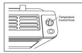
Push the temperature control knob onto the temperature control rod.
