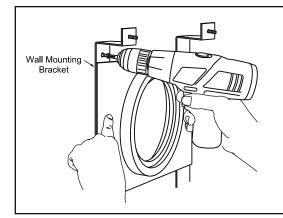
Using four (4) wood screws, attach the wall mounting bracket to the wall.
