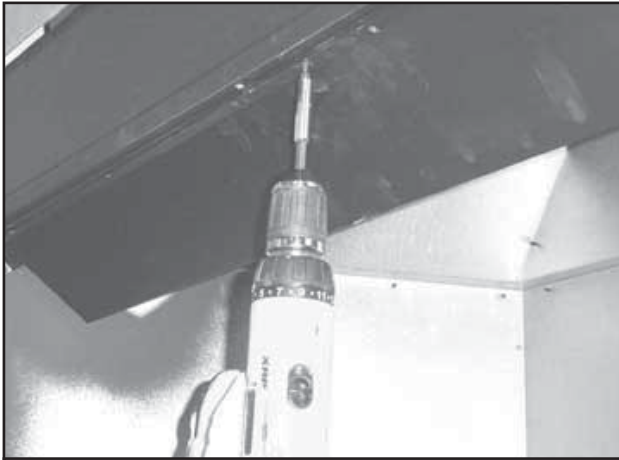
Figure 8.1 Remove Smoke Shield
