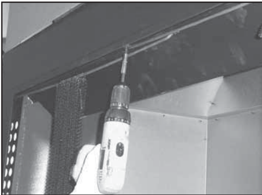
Figure 3.8 Remove Screen Rods
