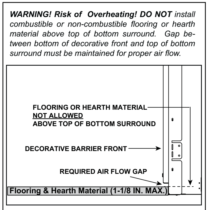
Figure 10.3 Required Air Flow Gap
