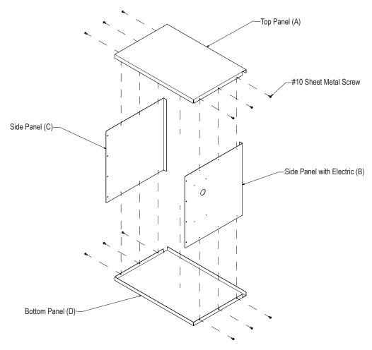
4. Position the assembled filter box on rear of furnace, supporting it approximately 4 inches from the floor, covering the rear distribution blower. Make sure the filter box is tightly pressed to the back of the furnace. Use 8 #10 self-tapping screws (included) to firmly attach the filter box to the sides of the furnace.
