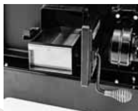
Ash Removal System
