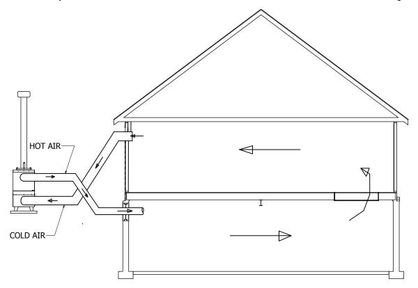
Outside Combustion air may be necessary for an indoor installation if:
