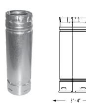
Features fully unitized, twist-lock construction in 3" and 4" diameters. Listed at 1" clearance to combustibles. It can be used in both vertical and horizontal installations. Stainless steel wall combined with a galvanized outer wall. Pipe OD is diameter plus %". Galvalume or painted black outer finish. 12" length available with stainless steel outer (SS).
