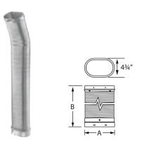
Use through damper and smoke shelf area. Use with DuraLiner Insulation Kit (ProMesh and ProFoil), where flex extends into clay liner, for zero-clearance applications. Built from 1-ply construction, .005" 304 stainless steel.
