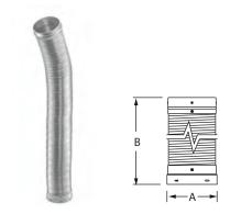
Use through damper and smoke shelf area. Use with DuraLiner Insulation Kit (ProMesh and ProFoil), where flex extends into clay liner, for zero-clearance applications. Built from 1-ply construction, .005" 304 stainless steel.
