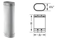
Use to reline masonry chimney with 0/0 clearance. Available in oval 6" and 8" diameters; 12", 24", 36", and 48" lengths. Factory-insulated. Built-in, pre-drilled fittings for riveting joints. 304 stainless steel inner and aluminized steel outer. Note: to calculate the installed length of 5", 6", and 8" DuraLiner pipe subtract 1 ½" from each joint overlap of liner pipe sections.
