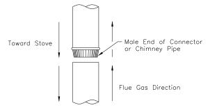
FIGURE 2.3 (A) Connecting Sections
