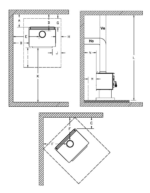
Figure 2: Clearances to combustibles and floor protector
