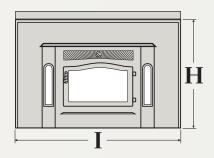
Special Notes: Crossfire must be installed on non-combustible surface (see installation manual).
