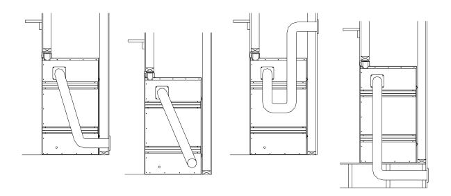
FIGURE 19: OUTSIDE AIR KIT INSTALLATION METHODS
