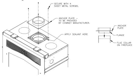
FIGURE 22: ANCHOR PLATE INSTALLATION
