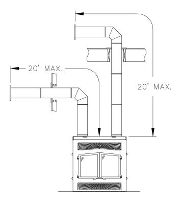
FIGURE 18: HOT AIR DUCT KIT MULITPLE LOCATION INSTALLATION
