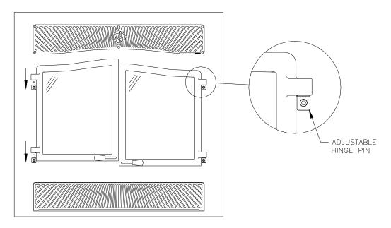
FIGURE 7: DOOR ALIGNMENT POINTS
