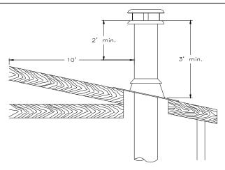
FIGURE 5: CHIMNEY INSTALLATION DIMENSIONS
