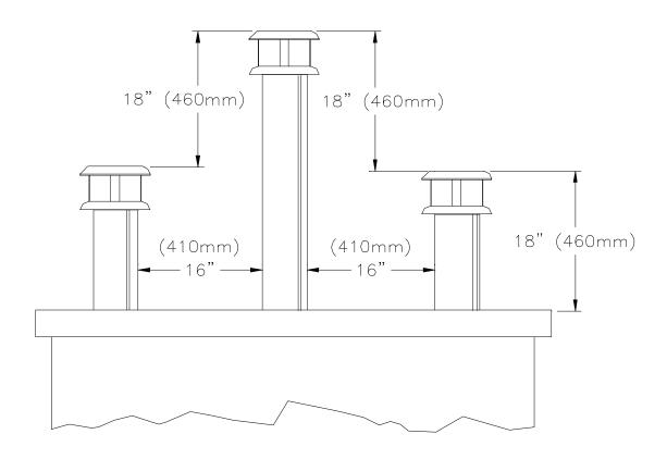
FIGURE 27: CHIMNEY CHASE AND MULTIPLE TERMINATIONS
