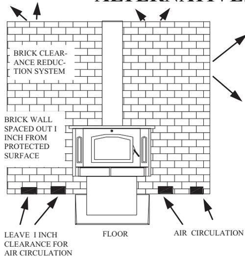
BRICK WALLS MAY BE ATTACHED TO COMBUSTIBLE WALLS USING WALL TIES IF BRICK IS USED. BE SURE FLOOR CAN WITHSTAND WEIGHT OF BRICK.
