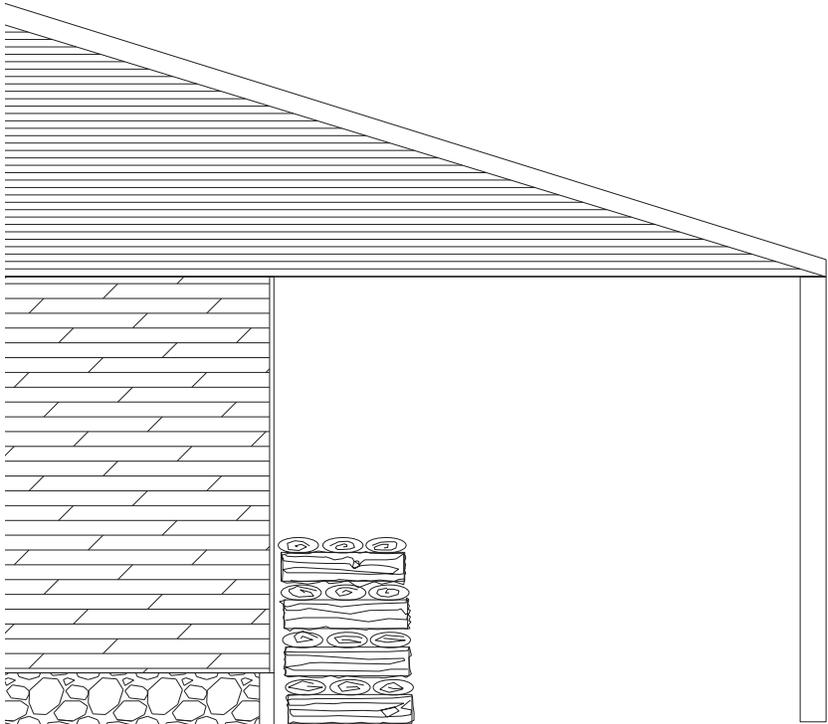
Stack wood in criss-cross pattern under a shelter to allow air flow to dry wood and to keep wood from rain. Green wood may have 50-60% moisture content. Wood seasoned outside uncovered may have 40% moisture content. Wood properly seasoned in a covered environment will have less than 20% moisture content.
