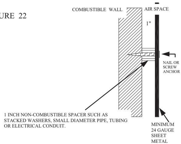
DO NOT USE FASTENERS DIRECTLY BEHIND CHIMNEY CONNECTOR OR STOVE.
