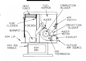
SIDE CUTAWAY - P2000FS
