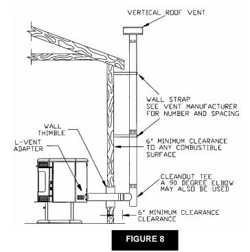
Locate terminations: a) not less than 3 feet above any forced air inlet located within 10 feet; b) not less than 4 feet below or horizontally from, or one foot above, any door, window or gravity air inlet into any building; c) not less than two feet from an adjacent building and not less than 7 feet above grade when located adjacent to a public walkway. Mobile home installations must use a spark arrester.
