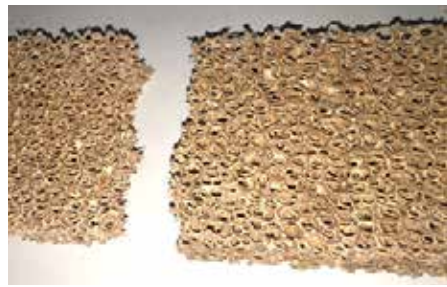
Combustor Problem - Broken Combustor
