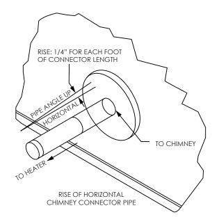
There are five allowable ways that a chimney connector can be connected to a masonry chimney by passing through a combustible wall. NFPA Standard 211 allows the following wall pass-through systems.
