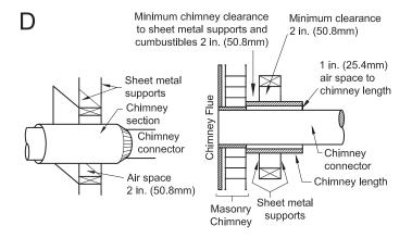
5. A listed factory-built wall pass-through system may be purchased and installed according to the instructions packaged with it to provide a safe method of passing the chimney connector through a combustible wall for connection to a masonry chimney.
