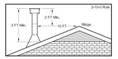
NOTE: Chimney height 3ft minimum (unless) any obstruction is 10ft or less away from the outlet then chimney height must be (X) pluse 2ft or the eft minimum, whichever dimension is greatest. X exquals height of obstruction. Masonry chimney shown dimensions are same for metal prefabricated chimney.
