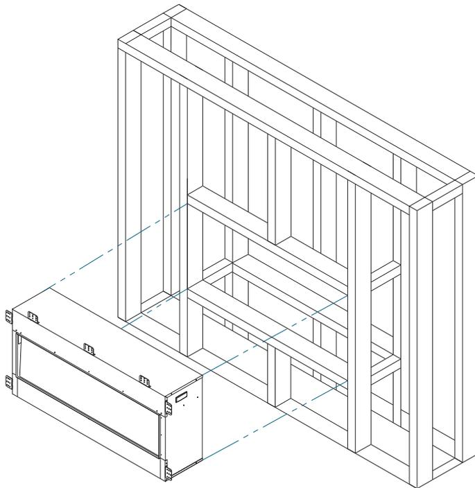
6. Drive the mounting screws into the framing plates on the unit and the wall studs.
