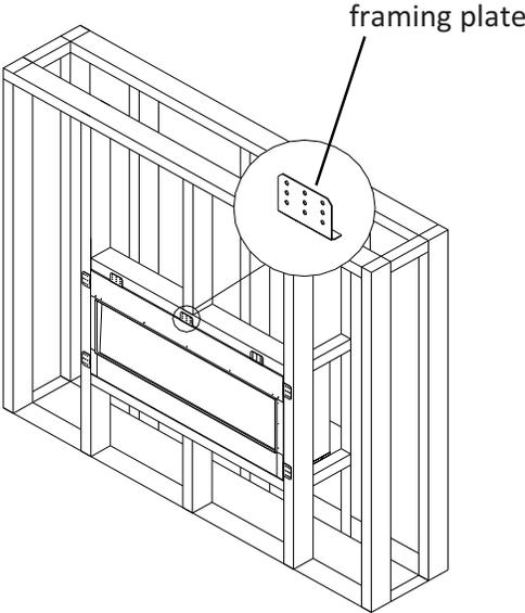
7. After checking that the fireplace operates properly, cover the glass panel with protective plastic bag and install plywood or drywall.
