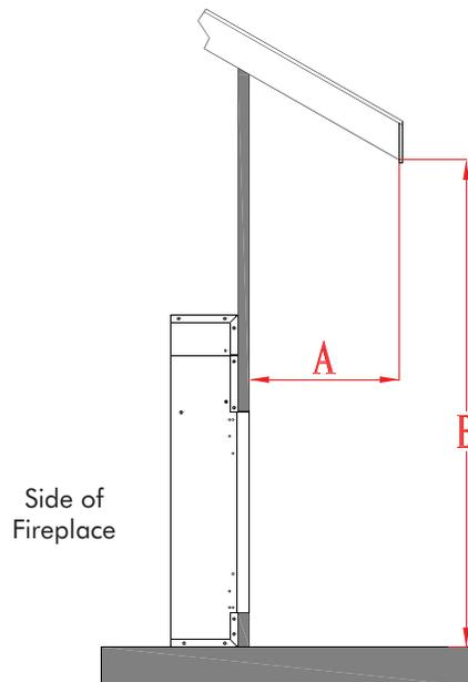
The overhang (A) must extend at least 1/2 the roof-line height (B). Height is measured from the base of the fireplace.
