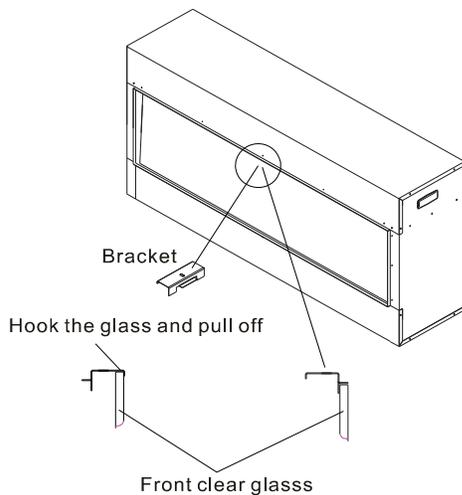
3. Put back the front glass and screw back the bracket.
