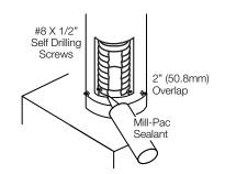
Always finish vent system installation with the appliance vent connection. Ensure that the sealant is not visible on the exterior pipes once installation is completed. An optional decorative black band may be available with this appliance. In the event that the venting must be disassembled, care must be taken to reseal the venting.
