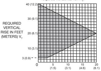
HORIZONTAL VENT RUN PLUS OFFSET IN FEET (METERS) H<sub>T</sub> The shaded area within the lines represents acceptable values for  $H_{\tau}$  and  $V_{\tau}$
