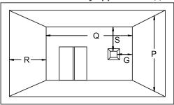
Q<sub>MIN</sub> = 3 feet R<sub>MAX</sub> ≤ 15 feet  $R_{MAX} = 2 x Q_{ACTUAL}$ (0.9m) (4.6m)
