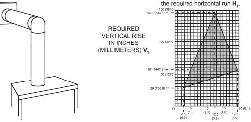
HORIZONTAL VENT RUN PLUS OFFSET IN FEET (METERS) H. The shaded area within the lines represents acceptable values for H<sub>+</sub> and V<sub>+</sub>
