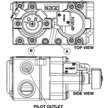
Prior to pilot adjustment, ensure that the pilot assembly has not been painted. If overspray or painting of the pilot assembly has occurred remove the paint from the pilot assembly, or replace. Fine emery cloth or a synthetic scrub pad (such as Scotch-Brite™) can be used to remove the paint from the pilot hood, electrode and flame sensor.
