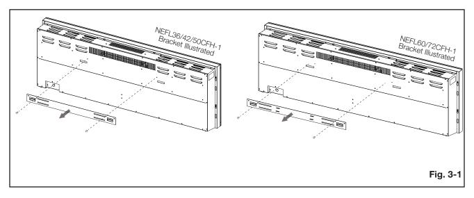
E. Mark out location, then mount the bracket onto the wall using screws (supplied). This bracket MUST have the hooks facing upwards and be level (Fig. 3-2i and Fig. 3-2ii, next page).
