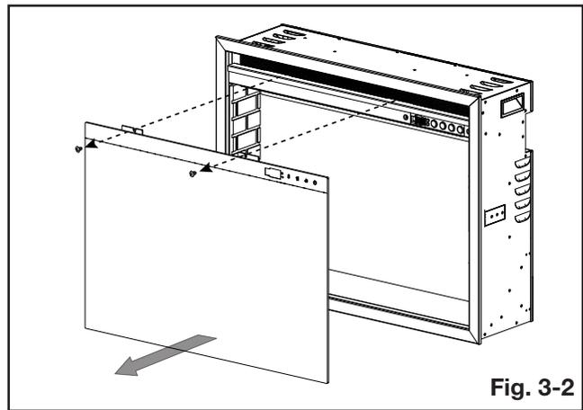
3. Remove all boxes packed inside the appliance (see "unpacking and testing appliance" section).
