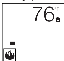
Flame at level 1
