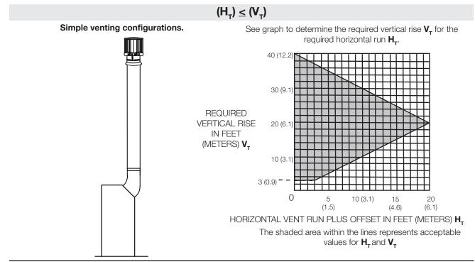
For vent configurations requiring more than one 45° and one 90° elbow, the following formulas apply: Formula 1:  $H_{\tau} \le V_{\tau}$ Formula 2:  $H_{\tau} + V_{\tau} \le 40$  feet (12.2m)
