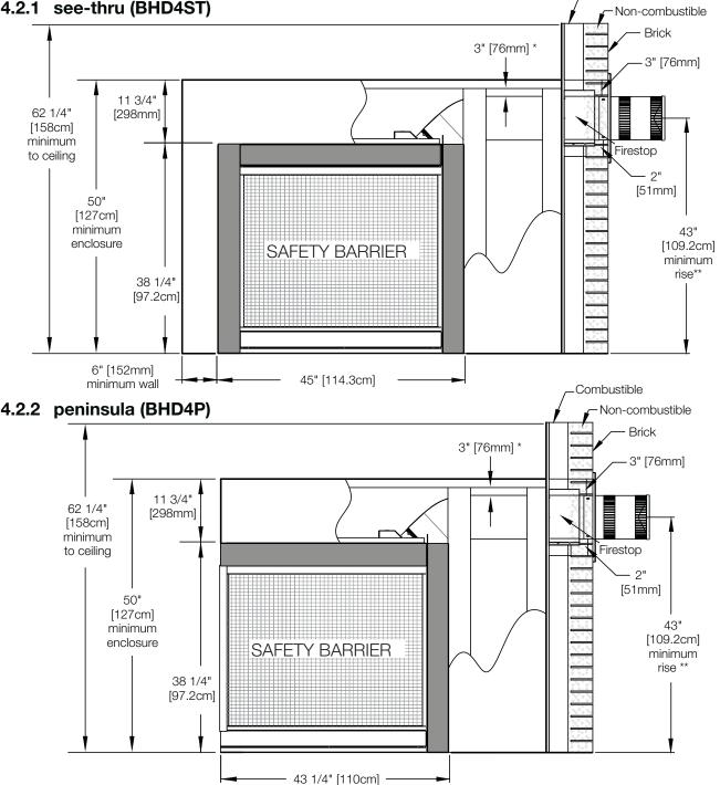
\* Within the appliance enclosure a minimum 3" (76mm) clearance between the top of the vent pipe and combustible materials is required. All other clearances within the enclosure, including where the vent pipe exits the enclosure are subject to 2" (51mm) to the sides and bottom and 3" (76mm) to the top for horizontal and 2" (51mm) for vertical.
