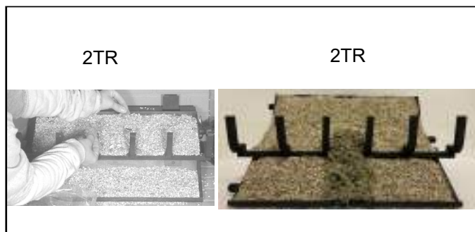
Figure 7.7 Rock Wool Placement
