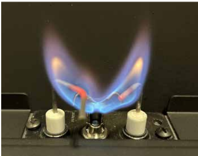
Figure 7.8 IPI Pilot Flame
