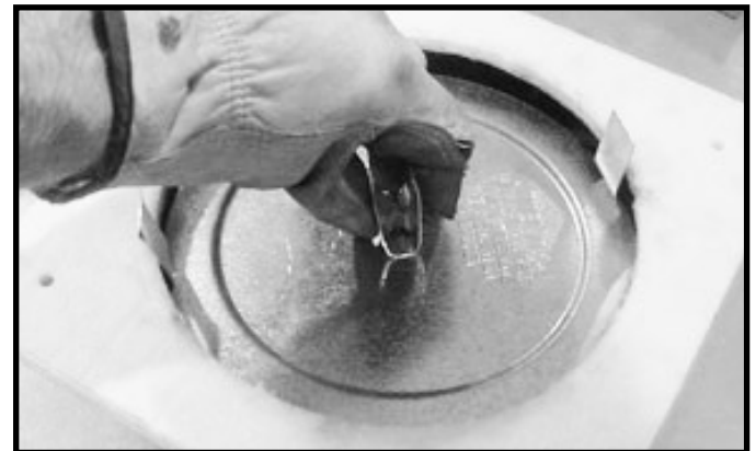
Figure 6.4 Fold the center parts of the retaining band up and use to remove the vent cap.
