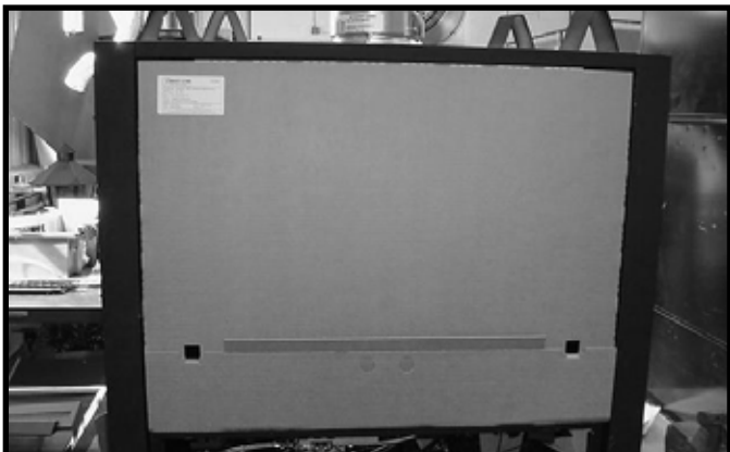
Figure 11.10 Splatter Guard with Lower Access Panel Open
