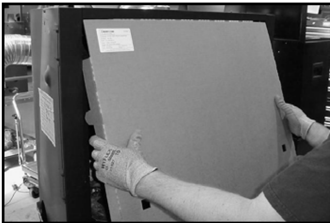
Figure 11.4 Installation of Splatter Guard
