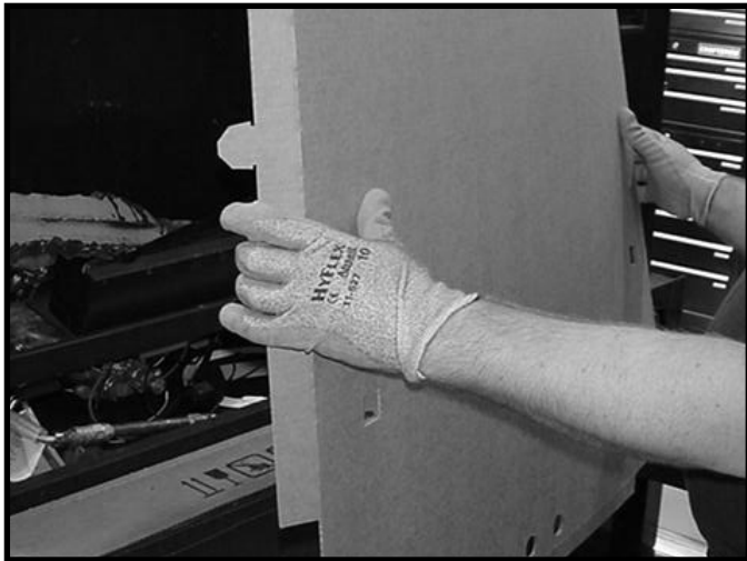
Figure 11.3 Folding of Right and Left Sides of Splatter Guard
