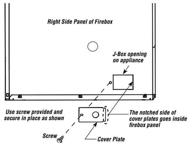
**Figure 22 - Installing J-box Cover Plate - All Models**
