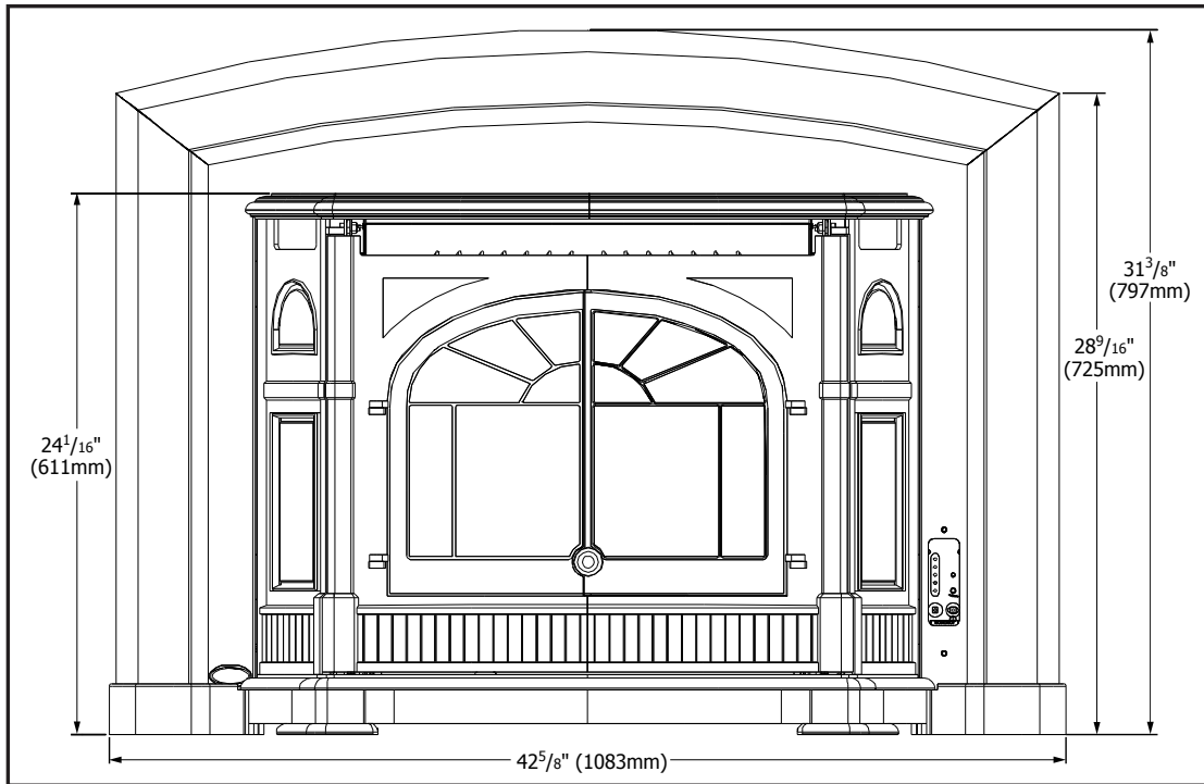
Figure 3: Dimensions of Empress Fireplace Insert with Optional Skirt.
